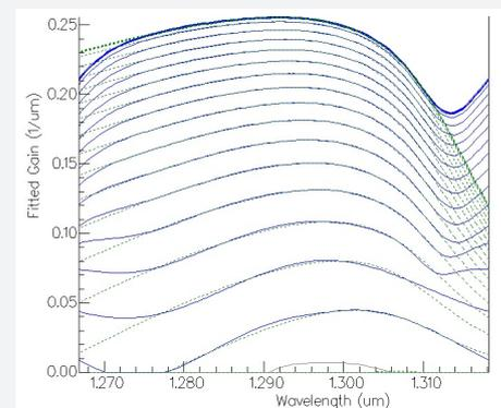
(above) Gain curves computed by Harold for a 3 QW InGaAsP epistucture are shown in green for different carrier densities. PICWave's fitted models are shown in blue. PICWave will import and fit almost all of Harold's other results, including spontaneous recombination, diffusion, refractive index data...
