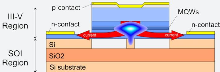
A hybrid silicon III-V laser with current spreading
