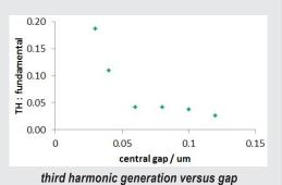
The graph to the right shows increasing power in the third harmonic as the gap is closed. This effect can form the basis of metamaterials with enhanced nonlinear optical response.
