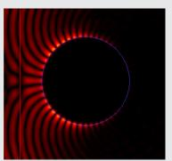
Mie scattering aroung gold sphere: field (high frequencies) and finite-elelement mesh
