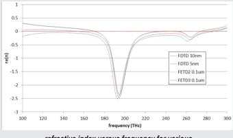
refractive index versus frequency for various FDTD and FETD resolutions: the negative index behaviour is shown below the red line
